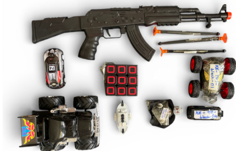
Photo 1: Toy gun with arrows (KE-toy-black-06-arrow) from the Kenyan market. This sample showed the highest total flame retardant burden of all analysed products, with total BFR concentrations reaching 188 mg/kg, dominated by DBDPE and BDE-209
